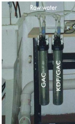
The diagram and picture on the left illustrate the apparatus designed to test the effectiveness of filters for bacterial control. A challenge water supply conforming to ANSI/NSF 42-1988 Standards feeds the filters, one containing a combination of KDF 55 process medium and carbon (KDF/GAC) and one containing carbon alone (GAC). The same water supply line feeds both filters. Two sets of filters were tested. The discharge lines for the
